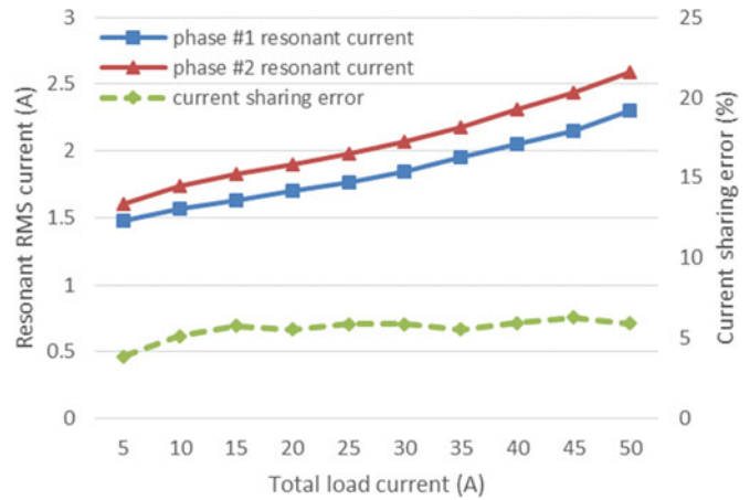
Fig. 22. Resonant current of the common capacitor two-phase LLC converter.
